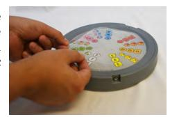
3. Install template by placing tabs in the slots as shown here. Make sure the red arrow points to the "ON" light. You can play song without overlay, but template may move and the position of the key can no longer be located by finger searching or touch.
