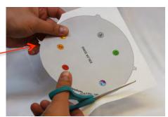
2. Remove plastic overlay that allows fingers to feel the area where keys are located. Take note that one of the tabs is smaller than the other tabs and must be placed in the slot near the octave changing switch when plastic overlay is replaced.
