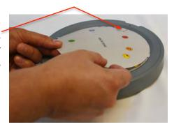
4. Replace plastic overlay. Make sure that the small overlay tab is in the slot near octave changing switch.
